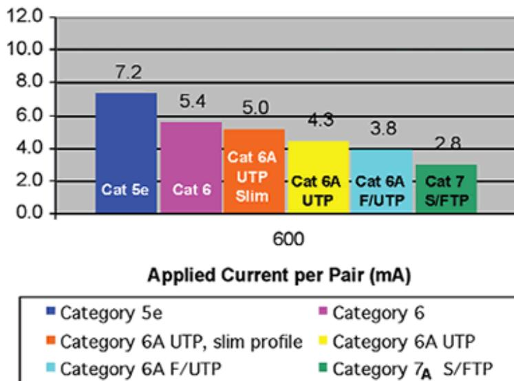
**Overview of the Siemon 100-Bundle Temperature Rise Versus APPLIED CURRENT Test Configuration:**
